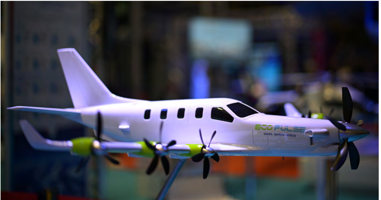
Illustration 2: Daher, Airbus and Safran team up to develop EcoPulseM, a distributed hybrid propulsion aircraft demonstrator. © Christel Sasso/CAPA Pictures.
