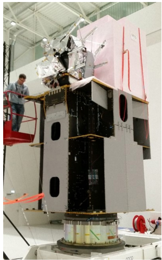
Fig. 5 Up: Sentinel-4 units location, configuration together with the IRS instrument on the MTG-S satellite. Bottom: Sentinel-4 STM mounted on MTG-S STM for the fit check (courtesy of OHB).
