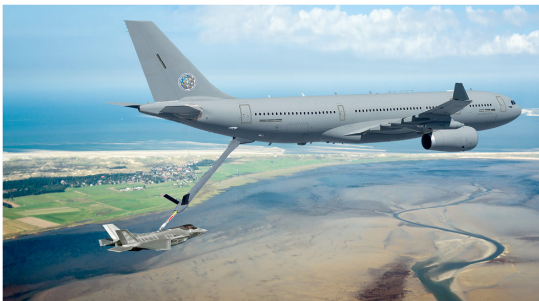
Air-to-Air Refueling sequence with an aircraft A330-200 MRTT
