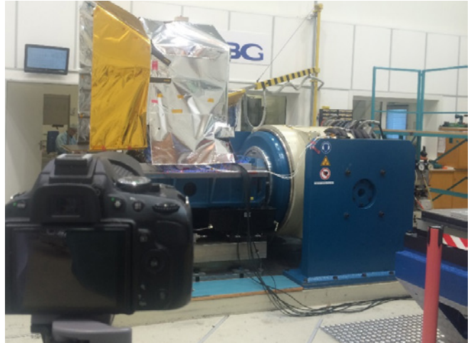
Fig. 12: OIM structure STM mounted on the vibration bench at IABG
