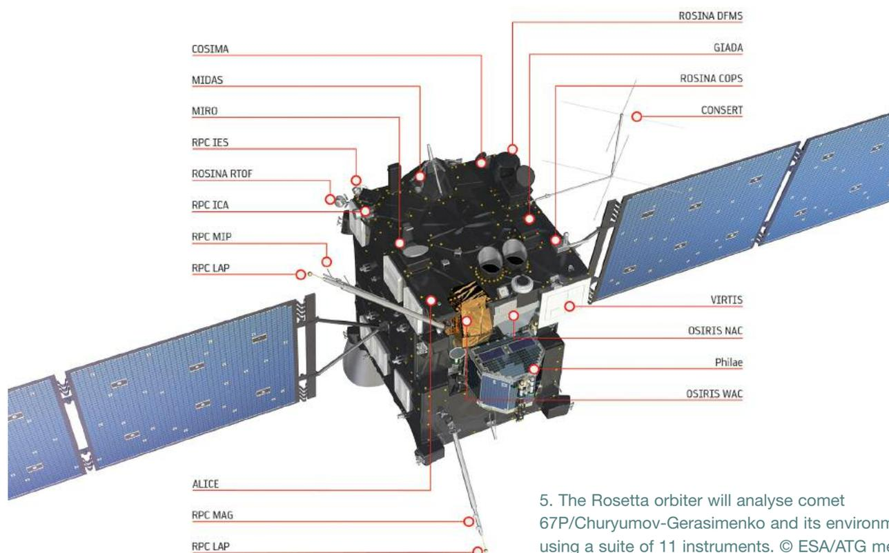
5. The Rosetta orbiter will analyse comet 67P/Churyumov-Gerasimenko and its environment using a suite of 11 instruments. © ESA/ATG medialab
